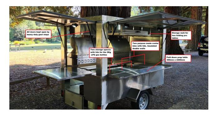
The barbeques are top quality and made of 304 Grade stainless steel. The two bbqs sits on a shelve that slides out 300mm to hang over the left side of the trailer. They are loose units and portable in other words the gas lines are not fixed to the body of the trailer at all
